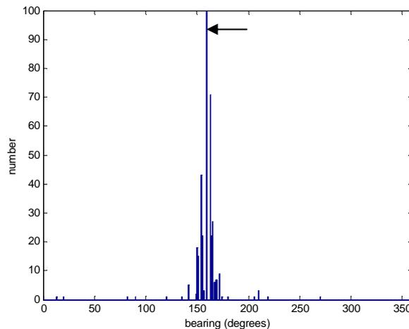
Figure 4. Histogram of bearings from position 1 (bearing used = 159°)
