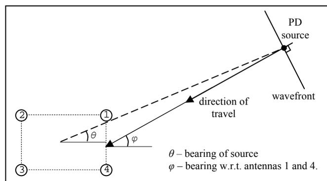
Figure 2. Relationship of bearing between two antennas and bearing with respect to the array.
