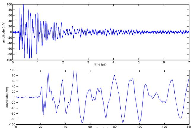
Figure 3. (a) Typical impulsive waveform originating from ABI (b) Wavefront of impulsive signal
